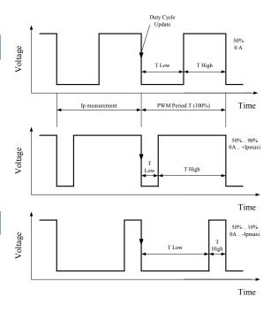
$$\begin{split} \textit{PWM period} \quad & T_{\textit{Period}} = T_{\textit{High}} + T_{\textit{Low}} \\ & \textit{PWM frequency} = \frac{1}{T_{\textit{Period}}} = 125 \textit{Hz} \\ & \text{DutyCycle(\%)} = \frac{T_{\textit{High}}}{T_{\textit{Period}}} \times 100 \\ & \text{DutyCycle(\%)} = 50\% + G \times I_{\textit{P}} \; \text{with G = Sensitivity (\%/A)} \end{split}$$
