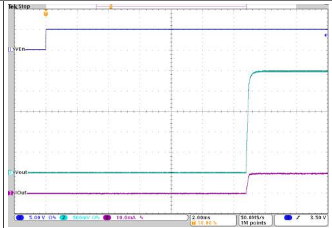
Figure 31. Startup with V_{OUT} = 2.5\text{ V}
