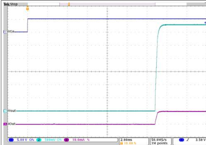
Figure 30. Startup with V_{OUT} = 3.3\text{ V}
